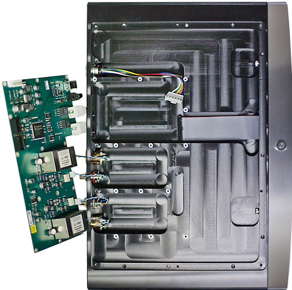
Fig. 4: Machined aluminum chassis with isolated pockets
